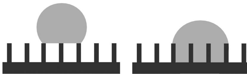
Fig. 1 A schematic illustration of the Cassie–Baxter state (left) and the Wenzel state (right).
